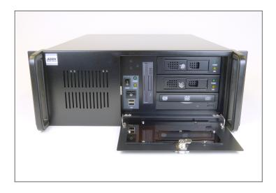
The AD-586E is an extended depth version of our extremely popular 4U system. This 4U industrial rack mount server can be configured for use with full size ATX server boards or with 14-slot backplanes. The extra depth allows for all expansion cards to be full-size (height and width). Multiple configurations are available for a variety of expansion slot requirements, whether you need ISA, PCI, PCIe, PCI-X or others, we can help.
