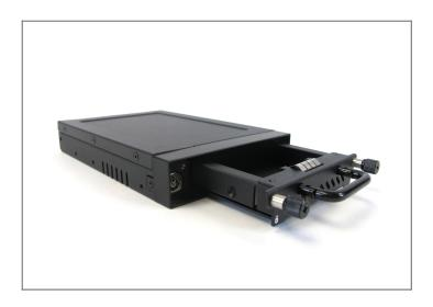
The 35-IS-BAY-B is a short depth 3.5" drive bay and removable carrier/tray for 2.5" SATA/SAS 6.0 Gb/s drives. This is a hot-swap cage built with durability in mind using aluminum and steel construction. Thumb screws keep the carrier in place, and an LED light features blue light to show hard drive power and red light for HDD accessing.
